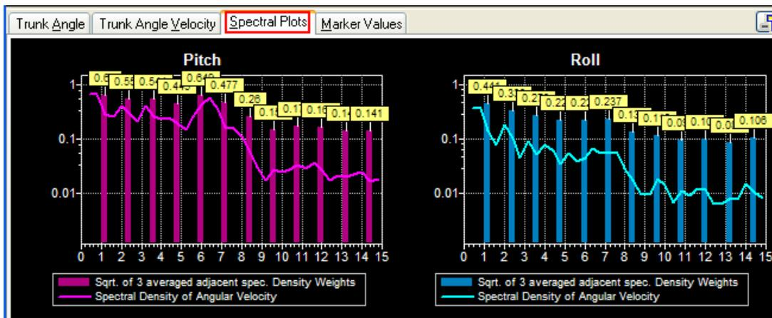
Spectral densities of pitch and roll angular velocities
