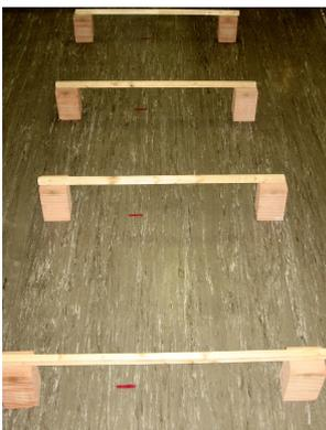
Construction bricks (about 21 cm high) and wooden slats (3 x 3 x 120 cm) can be used as shown here. When the wooden slats are laid across the bricks, they act as a barrier 24 cm high. Four such barriers should be used spaced 1 m apart.
