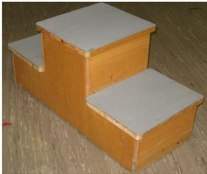
As shown on the left the set of stairs needs two upward and two downward steps with a step height of 23 cm, step depth 32 cm, step width 40 cm and preferably no handrails, but with non-slip plastic covering.
