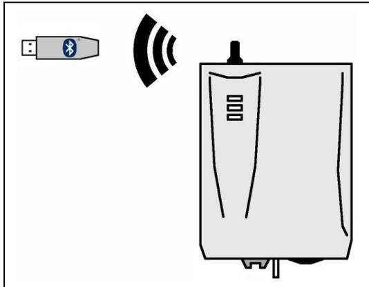
The **SwayStar™** hardware for connecting to the PC, is made up of the device itself and the Bluetooth® dongle (Figure 3). The data transfer occurs wireless.
